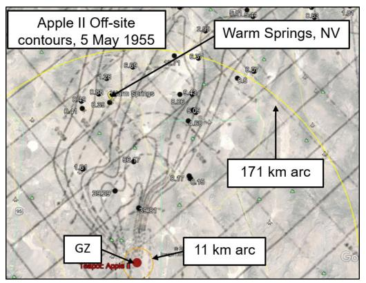
Figure 1. Summary of Apple II deposition pattern and pertinent geographic reference features. Map contours adapted from DNA 1979.<sup>5</sup>
