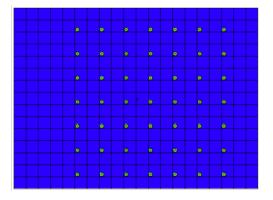
Fig. 3. Cross Section of 7 x 7 loading configuration with 10 cm pitch (left) and 20 cm pitch (right) modeled in MCNP. (Author produced drawing)
