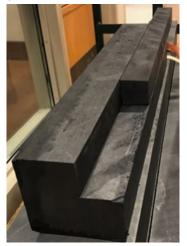
Fig 4. Experimental cut of graphite unit cell (Author picture) The machined graphite blocks can be manual configured as either of the two unit cellspr. Fig. 5 depicts unloaded and loaded unit cells near full insertion of a graphite moderating rod (left) and an aluminum cladding tube in which the uranium fuel will be contained (right).
