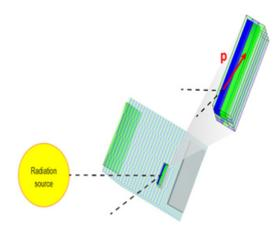
Figure 3. ASMM neutron detector design. Composed of alternating microscopic zones (50x50x50 microns) of scintillators small enough to give the detector sensitivity to the angle between a neutron-induced proton recoil and the long axis or "grain" of the zones. (J. Brodsky, 2020. Used with permission)
