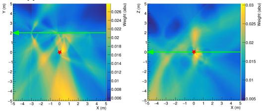
Figure 2. Left, modeled source localization with closest approach of 2 m. Right, modeled source localization with closest approach of 0 m. Modeling shows that source localization can achieved with similar accuracy. [2]
