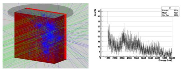
Figure 4. Left, GEANT4 side/top view of GSO:Ce crystal with 100 4.5 MeV neutrons interacting with the crystal face and a PMT located on the top plane. Right, GEANT4 output of the energy spectrum of a PuBe source incident on GSO:Ce of 50,000 events. [3]
