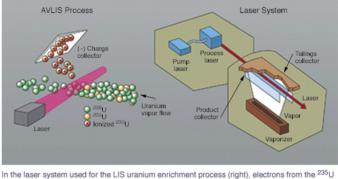
atoms are separated (left), leaving positively charged <sup>235</sup>U ions that can be easily collected for use. Figure 1: Simplified diagram of the AVLIS system [2]
